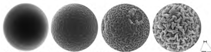
REM: different surface morphologies of carboxylated microspheres
