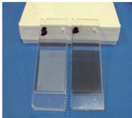
Retarded flow velocity of ink in unmodified (hydrophobic) channels
