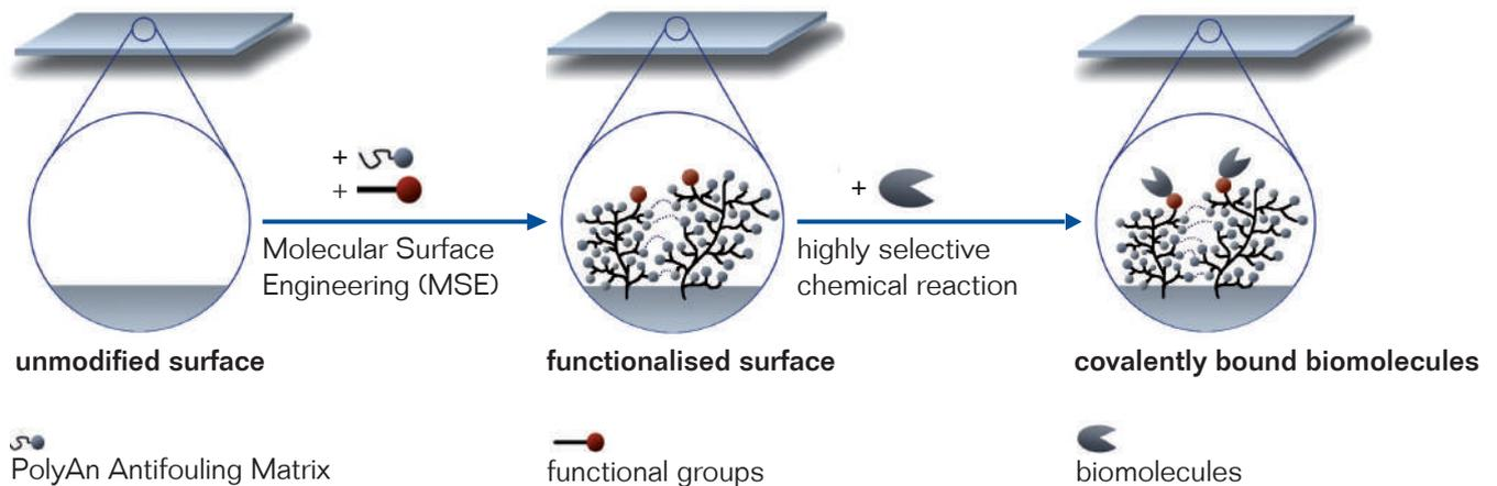
Our MSE-technology gently binds the functional layer onto the surface without damaging the base substrate. The morphology of the functional surface and thus the number of the reactive groups can be fine-tuned within a narrow range. This yields a number of advantages:
