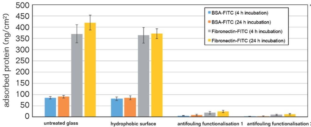
PolyAn's antifouling coating is covalently anchored on the base substrate. The surface modification is permanent. The autofluorescence and mechanical characteristics of the base substrate are not influenced by PolyAn's surface modification.
