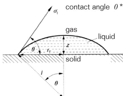
The contact angle is a measure of the wettability (hydrophilicity) of the surface. A narrow specification of the contact angle ensures uniform spot morphology (within a slide and from batch-to-batch) and can also be used as an indicator for the overall homogeneity of a surface.
